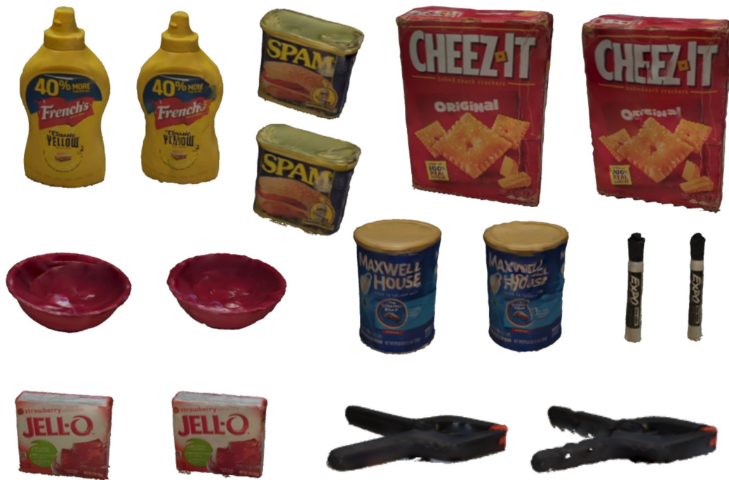
Figure 8: Reconstructed YCB-V objects, with the left/upper object illustrating reconstruction using 2DGS, followed by SVRaster.
